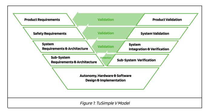
A high-level view of TuSimple's V Model is shown in Figure 1 above. Critically, the model enforces systematic end-to-end development of our autonomous platform by ensuring that:
