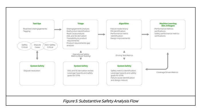
Figure 5 shows the high-level structure of our substantive safety flow. We begin with our test operations team reviewing and assigning tags to every single disengagement occuring during public road testing. Each disengagement is attributed with an abbreviated severity risk index. In some cases, our system safety team helps resolve disputed cases where test engineers may not easily be able to determine if the case would have been safety critical or non-safety critical.
