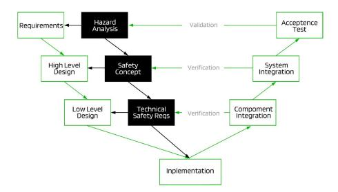
We follow the design V-diagram with the design creation from system to component on the left side of the V and the verification and validation from the component to the system on the right side.
