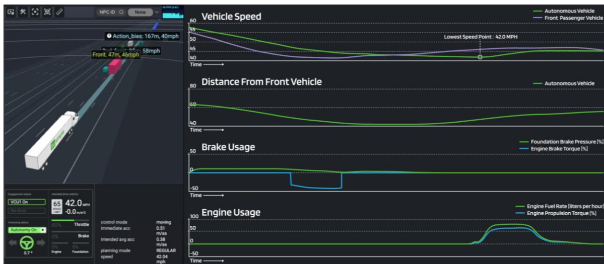
Figure 12 - Time Domain Behavior: Autonomous in Light-Traffic Scenario
